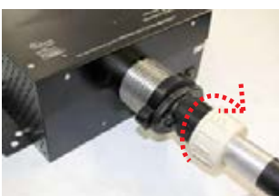
10) Screw on new fiber harness. (NOTE: It may be necessary to hold part to avoid twisting off)
